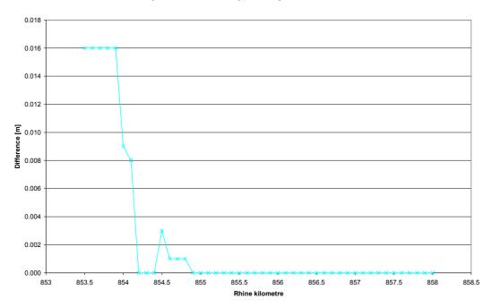
Figure 5-8: Differences in HHW between a scenario with forestation behind the first summer dike (see section 3.2) and the current situation
