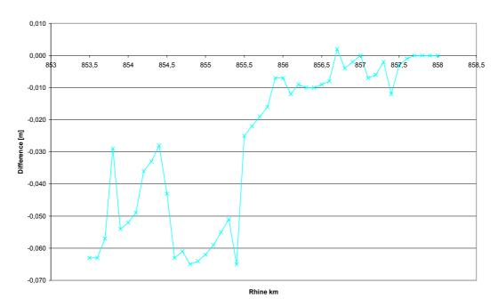
Figure 5-21: Differences in HHW between a scenario with a complete grassland coverage over the floodplain (see section 3.2) and the current situation
