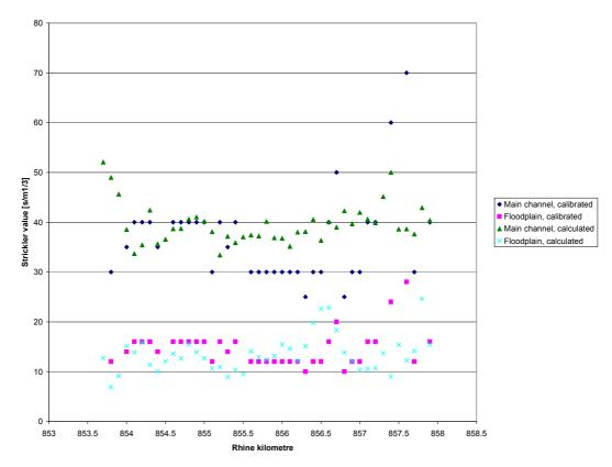
Figure 5-3: Calibrated and calculated Strickler values in main channel and floodplain
