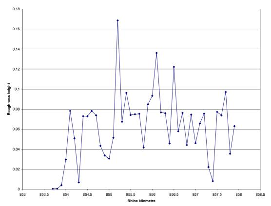
Figure 4-5: Calibrated floodplain roughness heights for each cross-section for the Rhine stretch along the Emmericher Ward
