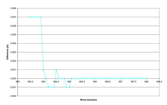
Figure 5-11: Differences in HHW between a scenario with forestation behind the second summer dike (see section 3.2) and the current situation
