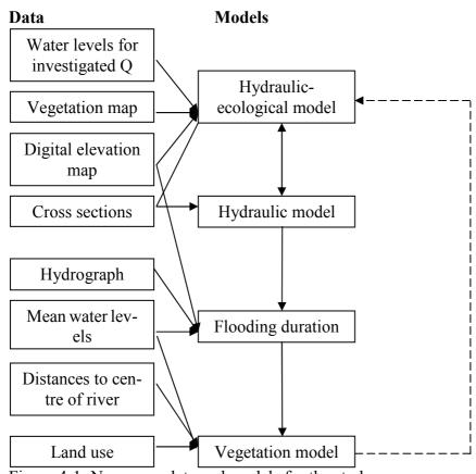
Figure 4-1: Necessary data and models for the study
