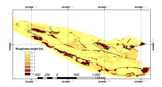
Figure 5-1: Roughness distribution over the floodplain during the HHQ of 1995
