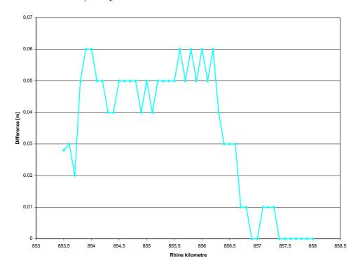
Figure 5-18: Differences in HHW between a scenario with complete coverage with PNV units and the current situation
