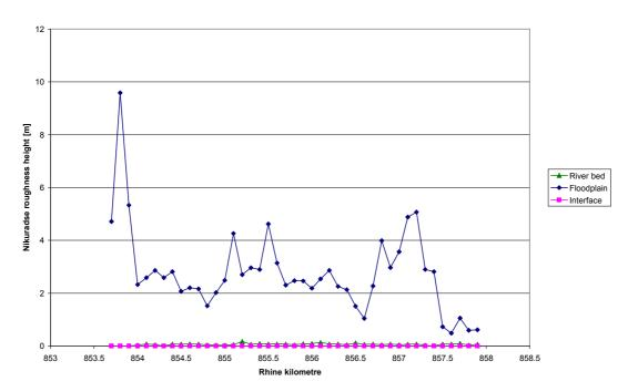
Figure 5-2: Roughness heights for each cross-section, current situation, HHQ of 1995
