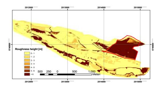
Figure 5-9: Roughness distribution over the floodplain, forestation behind the second summer dike (see section 3.2), HHQ of 1995, the red line shows the boundary of the forestation
