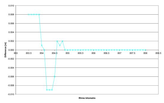
Figure 5-6: Differences in HHW between a scenario with forestation of all three areas (see section 3.2) and the current situation
