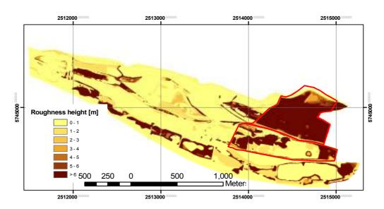
Figure 5-12: Roughness distribution over the floodplain, forestation in clusters between both summer dikes (see section 3.2), HHQ of 1995, the red line shows the boundary of the area in which forestation clusters are planned
