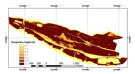
Figure 5-16: Roughness distribution over the floodplain in case of a coverage with PNV units, HHQ of 1995
