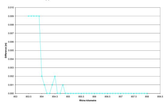
Figure 5-14: Differences in HHW between a scenario with forestation in clusters between both summer dikes (see section 3.2) and the current situation
